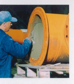
Internal cementlining of pipesystems protects the inner steel surface from corrosion and provides excellent hydraulic properties.
