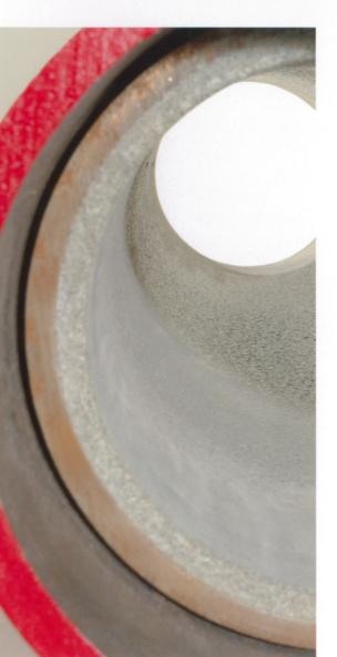
Cementlining in the field or in stockyard with special designed equipment is done by Conpipe in cases where renovation of an existing pipeline is required or for economical reasons. Handling and transportation of large bore above 1200 mm cementlined pipes may cause damage to the lining.
